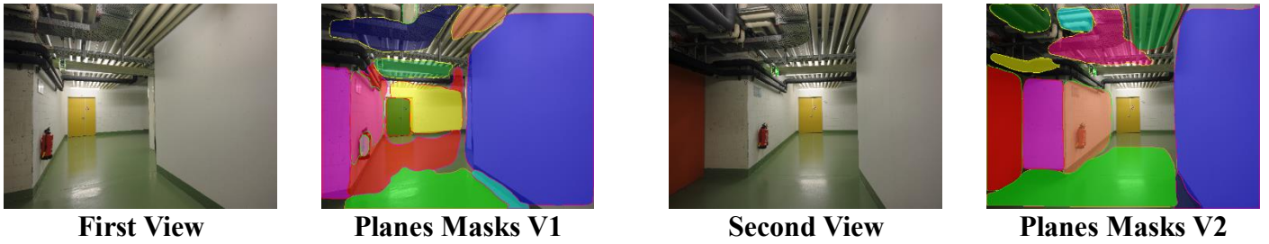
Figure 4.3(a): Plane Mask for neighbouring views in pipes scene left to right: first view, plane masks v1, neighbouring view, plane masks of neighbouring view.
