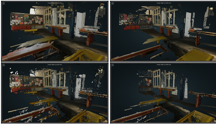
Fig. 10 Qualitative results from the lounge dataset from the high resolution test data. Top left: DeepPCF-MVS. Top right: PCF-MVS. Bottom left: TAPA-MVS. Bottom right: ACMM.
